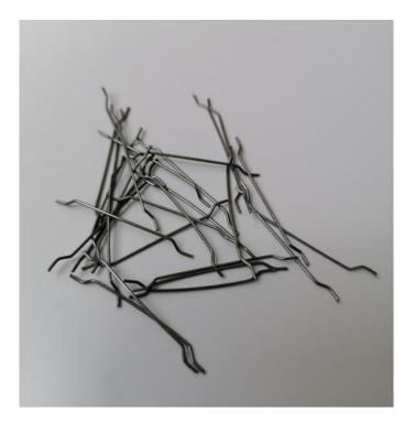
This kind of steel fiber is a high-performance steel fiber, which can improve the impact resistance and fatigue resistance of concrete; improve the impermeability of concrete. Because of its high tensile strength, good toughness, and low price, it is often used as a substitute for steel fiber.
